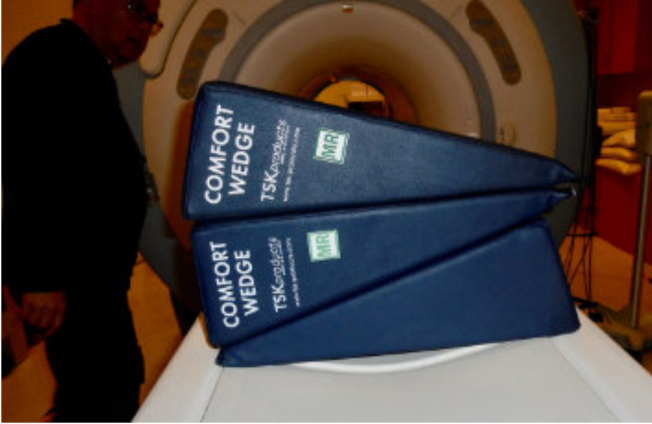
Comfort Wedge with digital printing that underwent MRI at 3-Tesla and the MR images that were obtained, shown below.
